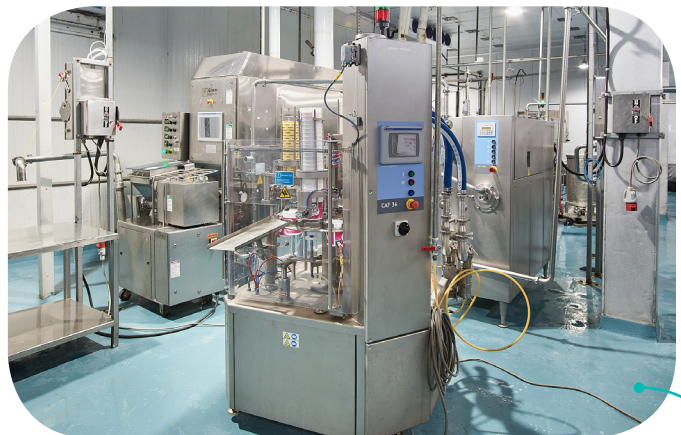
The new automatic filler used in the filling of quarts and pints of Kremi Ice Cream.
