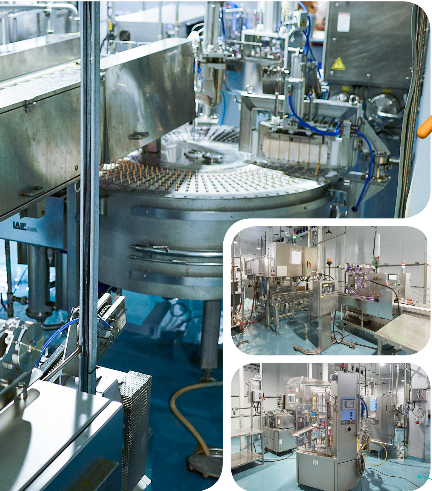
The new automatic filler used in the filling of quarts and pints of Kremi Ice Cream.
